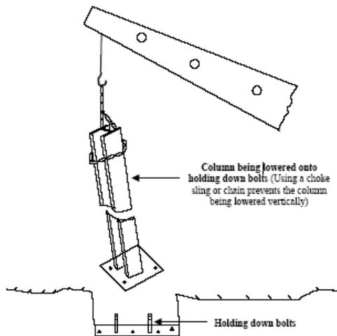
Problem: Steel column sections were lifted into place using a crane. A choke sling was used as the attachment method. Manual handling of the steelwork was required to attach the sling. Once suspended, the column did not hang vertically. Manual handling was therefore required to correctly position the column on the holding down bolts. Once in place a worker needed to use a ladder or 'cherry picker' to remove the sling.
